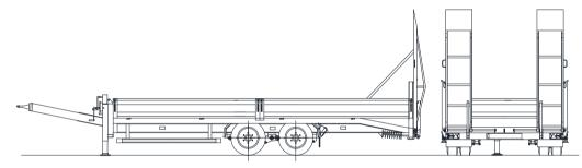
Axles: Gigant high-speed axles with maintenance-free parabolic spring unit, S-cam brake and load compensation
