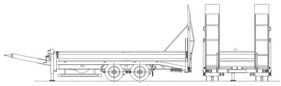
Axles: Gigant high-speed axles with maintenance-free parabolic spring unit, S-cam brake and load compensation
