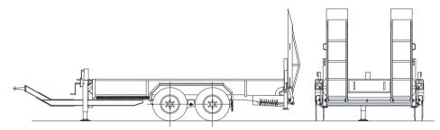
Axles: Fast-running axles type BPW, with a maintenance free parabolic spring assembly, cam brakes and weight adjustment
