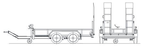
Axles: Knott fast-running axles with leaf springs, cam break and weight adjustment
