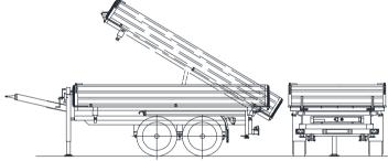
Axles: Fast-running axles type Gigant with maintenance-free parabolic spring assembly and weight adjustment
