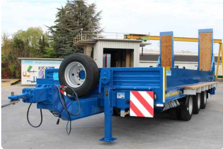
Tridem 25t TW with insertable side walls made of aluminium, width extendable to 3,0m, warning package (with a connector and holder for a rotating beacon as well as illuminated extendable warning sides) and spare tyre
