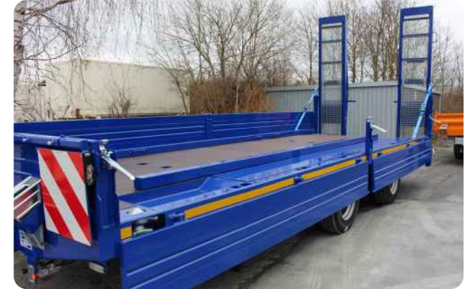
Combo-transport trailer: suitable for the transport of roll-off containers and construction machinery - with insertable guide for the roll-off containers
