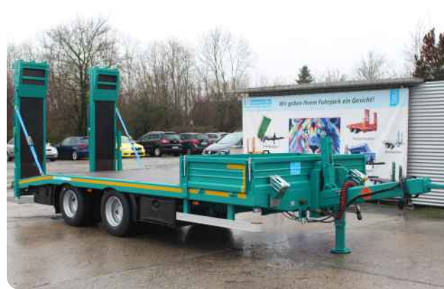
Special rubber surface in the ramps and bevel, ramps extended and foldable, divided front loading area with detachable sidewalls and border
