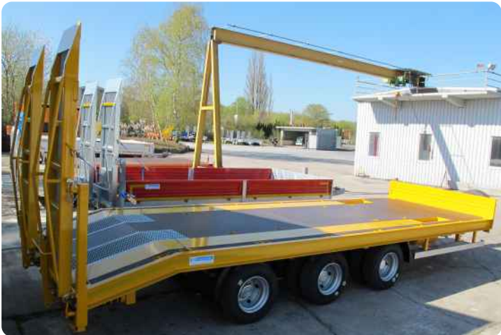
Tridem 25t TW, as a combo-trailer for the transport of roll-off containers and construction machinery
