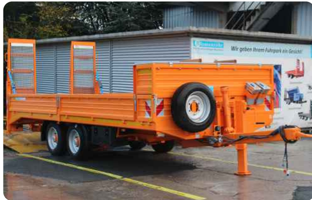
Double storage case - below with sideways flaps and an aluminium flap for the loading from the top, hardwood on the flap for the excavator shovel, widened ramps, divided side walls, spare tyre and net hooks
