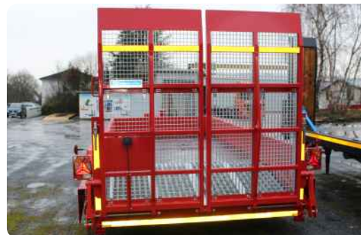
Closed loading ramp, with slide protection grids at the slope
