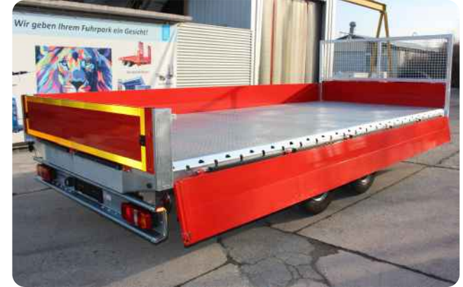
Chassis hot-dip galvanized, outer profile with double hole pattern, aluminum side walls 400mm high, elevated front wall made of corrugated mesh, steel plate floor
