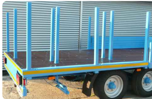
Stanchions can be plugged in at specified the position, with steel side walls on the front half of the loading area
