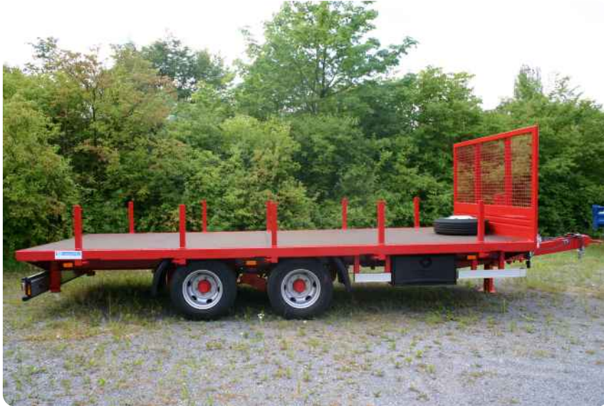
With plug-in stanchions on the side, tool box and front wall elevation made of corrugated wire mesh
