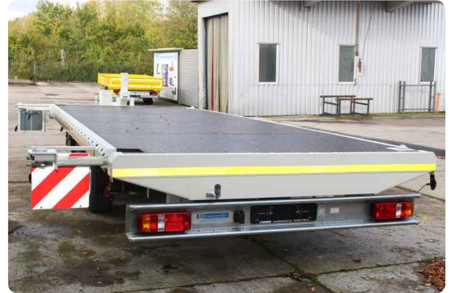
As a platform trailer for container transport with telescopic container locks and warning package (extendable, illuminated warning signs, connector for rotating beacon)
