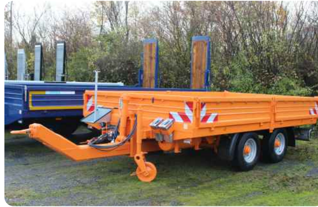
Model 745/5000: with support wheel, steel sidewalls, net hooks, warning signs, holder for traffic cones, divided sidewalls
