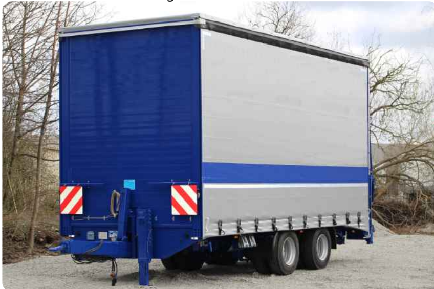
With sliding tarpaulin body, front wall made of aluminum profiles, warning package (extendable, illuminated warning signs)
