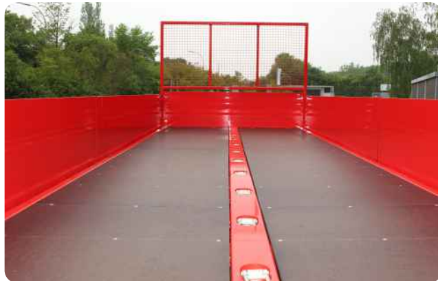
Central lashing rail with rotatable lashing troughs, 4000 daN load capacity
