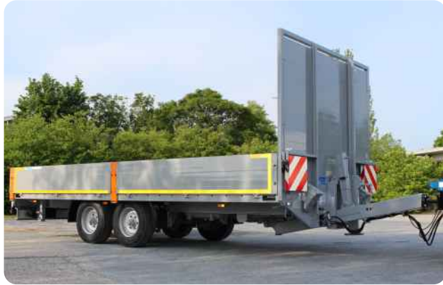
500mm high aluminium sidewalls, divided, with front elevation up to 2m height, with warning package (lighted warning signs, connector for rotating beacon), twist locks, air suspension
