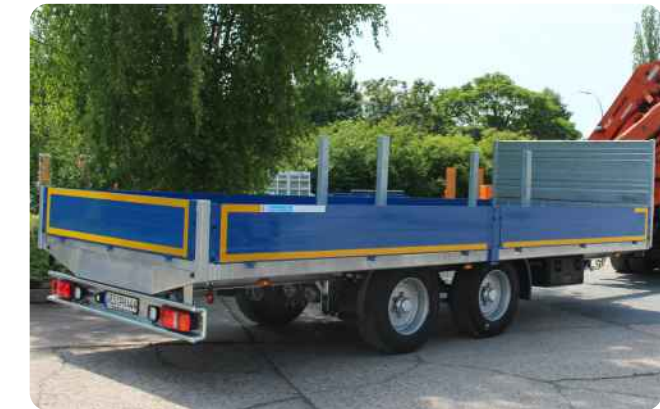
Hot-dip galvanized chassis, increased steel front wall to 80 cm, stakes can be plugged in at the desired position, additional LED reversing lights, divided side walls
