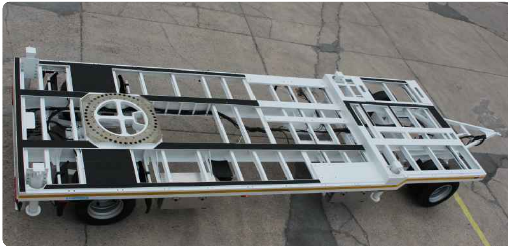
Also possible as a two-axle chassis with special connection or supports
