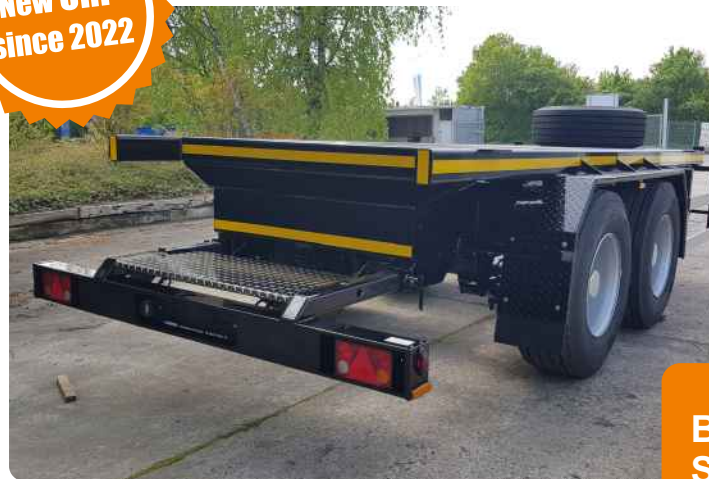
With extendable underrun protection (can only be delivered with TÜV homologation)
