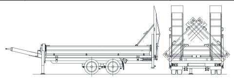
Axles: Fast-running axles type BPW with cam brakes, maintenance-free parabolic spring assembly and weight
