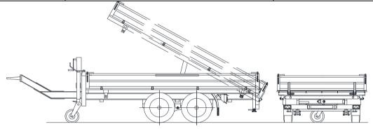
Axles: Fast-running axles by Knott with cam brakes, leaf spring and weight adjustment
