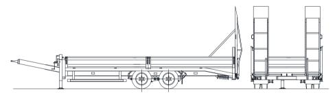
Axles: Fast-running axles type Gigant with cam brakes, maintenance-free parabolic spring assembly and weight
