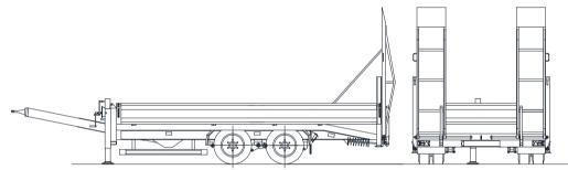
Axles: Fast-running Gigant axles with cam brakes, maintenance-free parabolic spring assembly and weight adjustment
