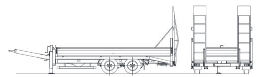
Axles: Fast-running BPW axles with S-cam brakes, maintenance-free parabolic spring assembly and weight adjustment
