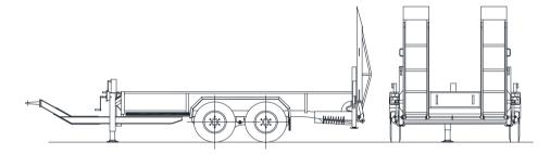
**Axles:** Fast-running axles type BPW, with a maintenance free parabolic spring assembly, cam brakes and weight adjustment
