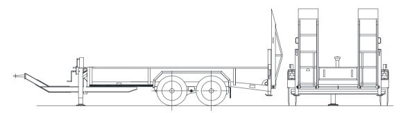
Axles: Fast-running axles type GFA, with cam brakes, leaf springs and weight adjustment
