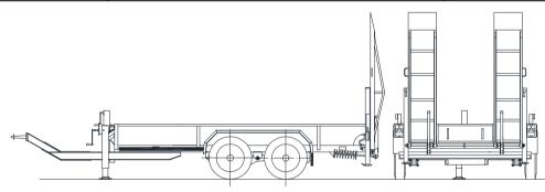
Axles: Fast-running BPW axles with a maintenance free parabolic spring assembly, cam brakes and weight
