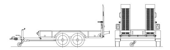
Axles: Maintenance-free rubber spring axles with precision bearings
