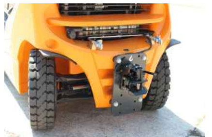
Yellow/red couplings mounted close to the hitch
