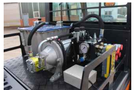
Two circuit hydraulic aggregate
