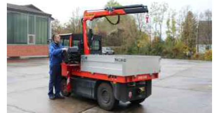
Crane PC1500 installed with sidewalls
