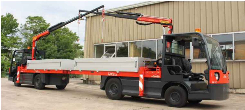
Crane PC1500 installed with sidewalls
