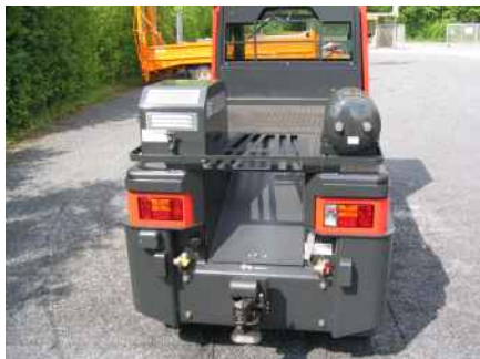
Pneumatic connectors „Standard“ (yellow/red air plugs)
