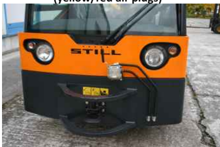
Pneumatic line also at the front
