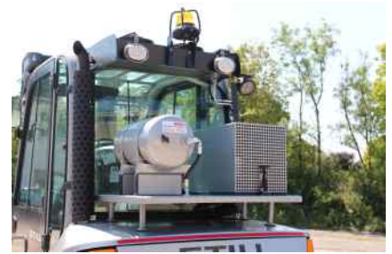
Compressor and tank mounted on a base plate, the rear view is guaranteed
