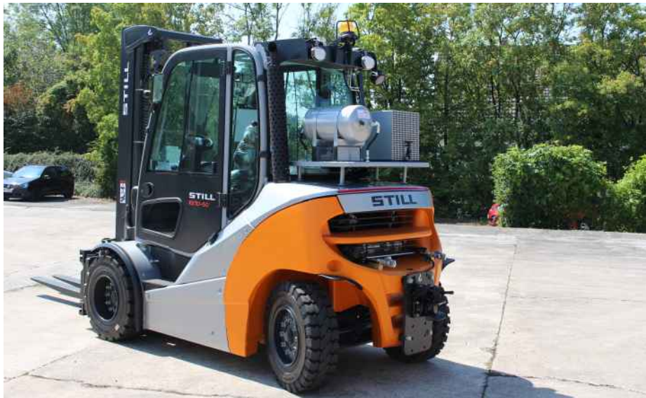
Yellow/red couplings mounted close to the hitch
