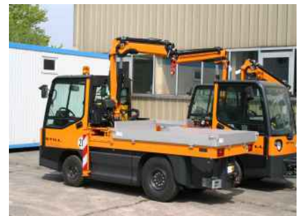
Crane PC1500 with low sidewalls
