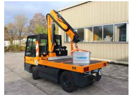
Crane PC2700 installed without sidewalls
