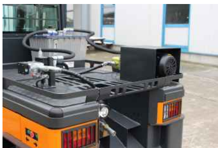
Single circuit hydraulic aggregate
