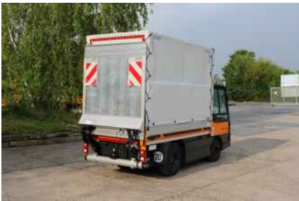
BÄR tail lift mounted at rear
