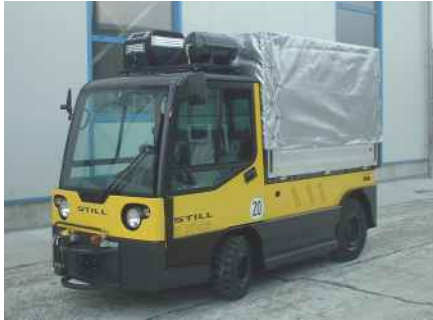
Air brake system mounted on the roof
