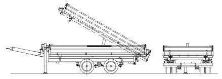
Axles: Fast-running axles type Gigant with cam brakes, maintenance-free parabolic spring assembly and weight
