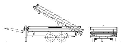
Axles: Fast-running axles type BPW with cam brakes, maintenance-free parabolic spring assembly and weight
