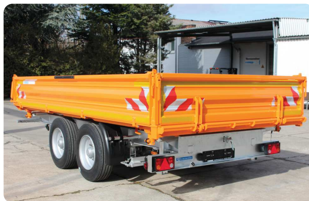
Model 863/8900 (Model 852/6900 similar) with warn markings, spring lifters, galvanized chassis - in serial equipment approx 6,45t PL
