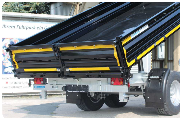
Tailboard as double wing door instead of oscillating flap, net hooks, big tyres, galvanized chassis and net hooks
