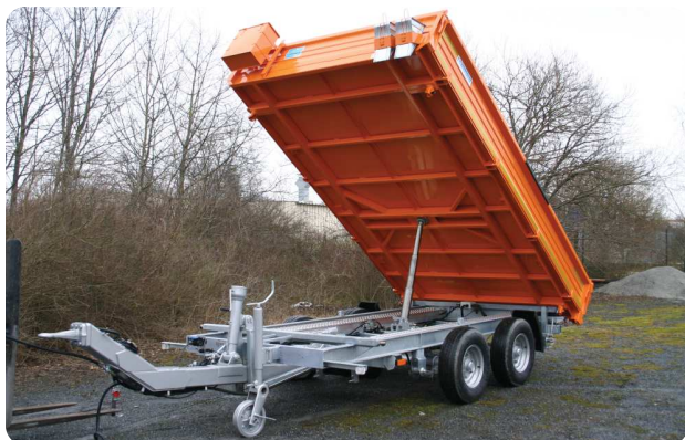
Model 845/5000 with tool box and galvanized chassis - in serial equipment approx 3,1t PL
