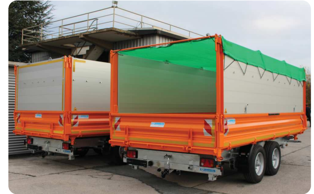
Superstructure for chaff, approx 1,20m high, made of anodized aluminium side walls with tarpaulin and additional car coupling at the rear
