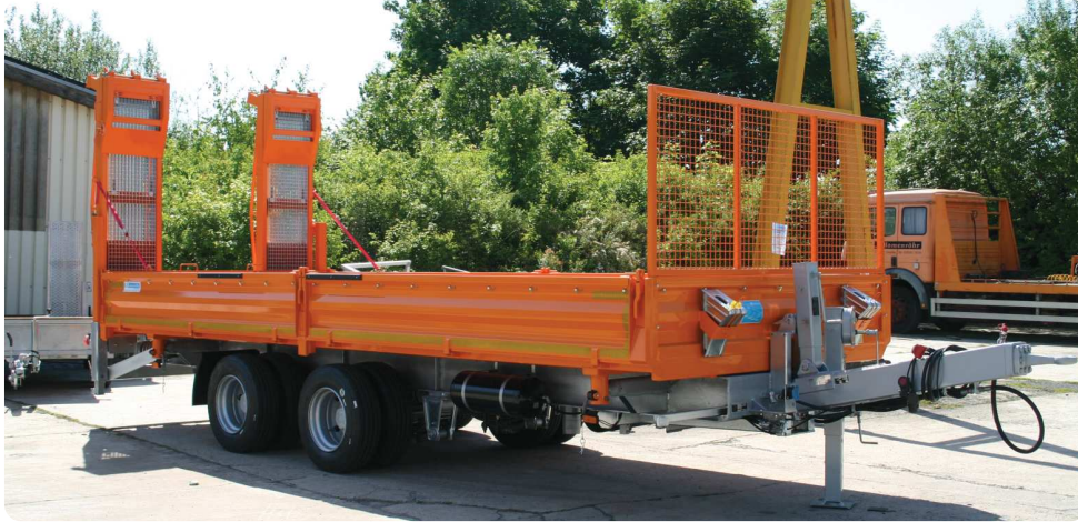
Front wall elevation made of corrugated wire, ramps extended and divided, galvanized chassis, divided sidewalls, grids in the ramps, net hooks
