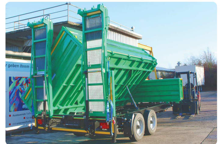
With additional steel sidewalls, double storage box, divided ramps, grids in the ramps and hydraulic ramp lifters
