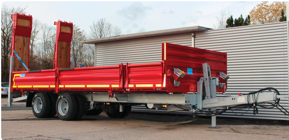
Additional loading platform at the front (not tipping), with elevated front wall, divided sidewalls and divided ramps
