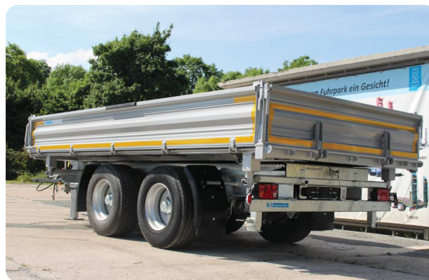
Model 888/14000 with tyres 385/55 R 19,5, spring lifters and galvanized chassis, sidewalls 50cm high - in serial equipment approx 11t PL
