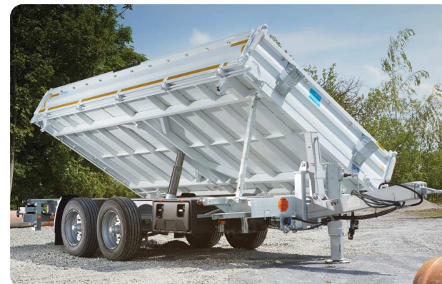
Model 885/10500 (Model 884/11900 similar) with net hooks, spring lifters, tool box, galvanized chassis, central locking system - in serial equipment approx 7,8 or 9,2t PL
