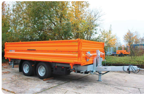
Additional steel walls, galvanized chassis, net hooks, central locking system
