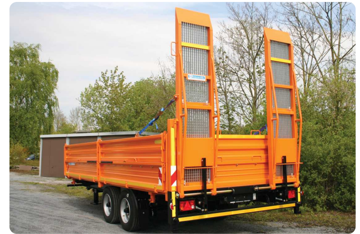
Additional sidewalls made of steel, divided sidewalls and additional side walls, grids in the ramps
