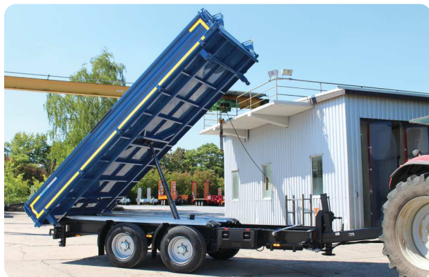
Model 888/14000 with tyres 285/70 R 19,5 extended to 5,50m loading area - in serial equipment approx 11t PL
