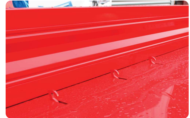
Lashing hooks with 4000daN lashing capacity in the tipper floor
