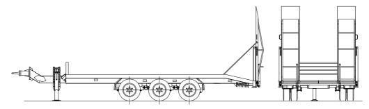
**Axles:** Type Gigant Axles with S- cam brakes, maintenance-free parabolic spring assembly and weight adjustment
