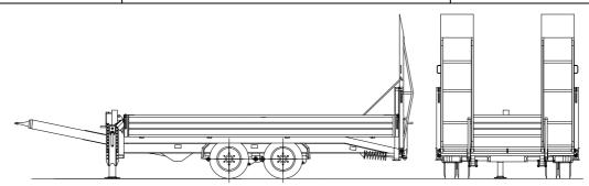
**Axles:** Fast-running BPW axles with cam brakes, maintenance-free parabolic spring assembly and weight adjustment
