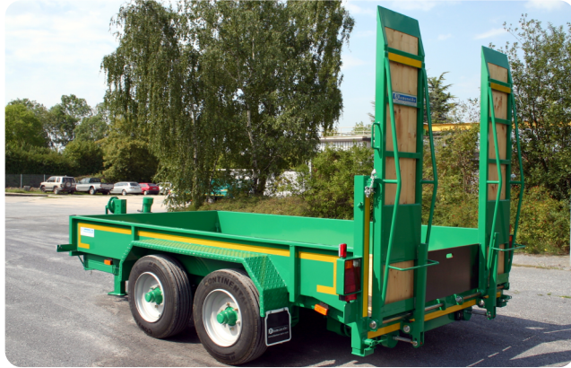
AWST 566/8900 with spring lifting supports
