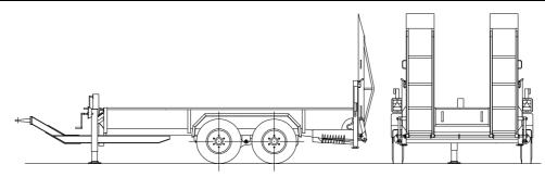
**Axles:** Fast-running axles type BPW, with a maintenance free parabolic spring assembly, cam brakes and weight adjustment
