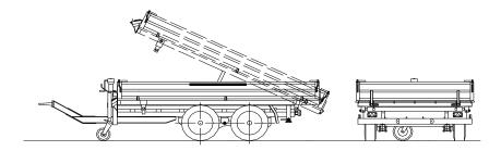
**Axles:** Fast-running Knott axles with cam brakes, leaf spring and weight adjustment
